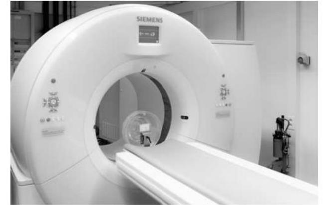
Fig.4 Hybrid CT scanner equipped with both CdTe counting detector and conventional GOS-based energy integrating detector.
