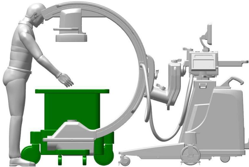
Figure 3. Theoretical position of surgeon while operating on a patient if steel counterweights are used. This is impossible as the edge of the C-arm prevents the surgeon from standing over the patient and so they would not be able to view them properly
