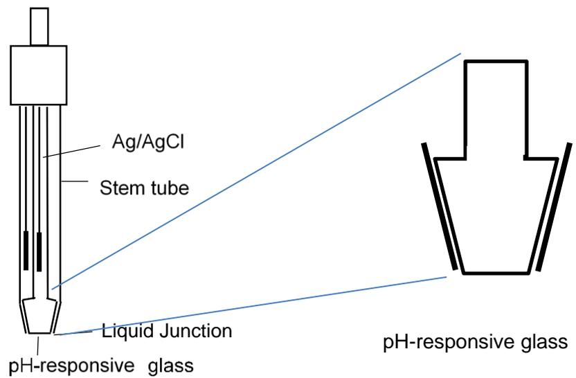
Figure. 3 Flat type example configuration
