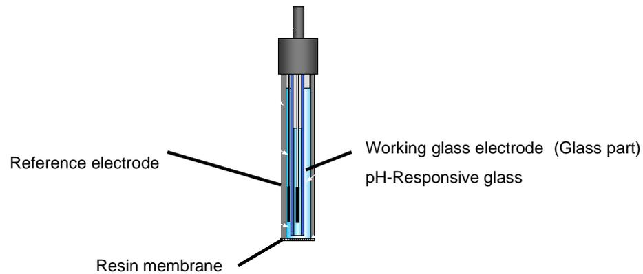
Figure 2 Configuration example of ion-selective electrode equipped with a pH glass electrode
