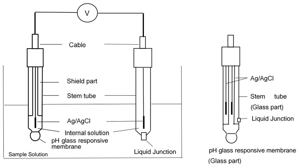
**Figure.1 Configuration example of a pH electrode**
