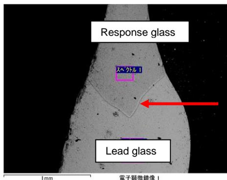
Figure 7 SEM photograph of the joint between lead glass and pH response glass showing the diffuse interface layer
