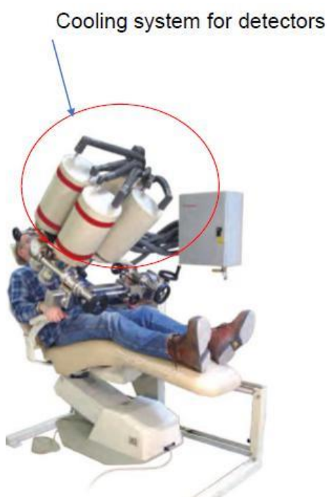
Figure 4-6: Lung counter with a cooling system
