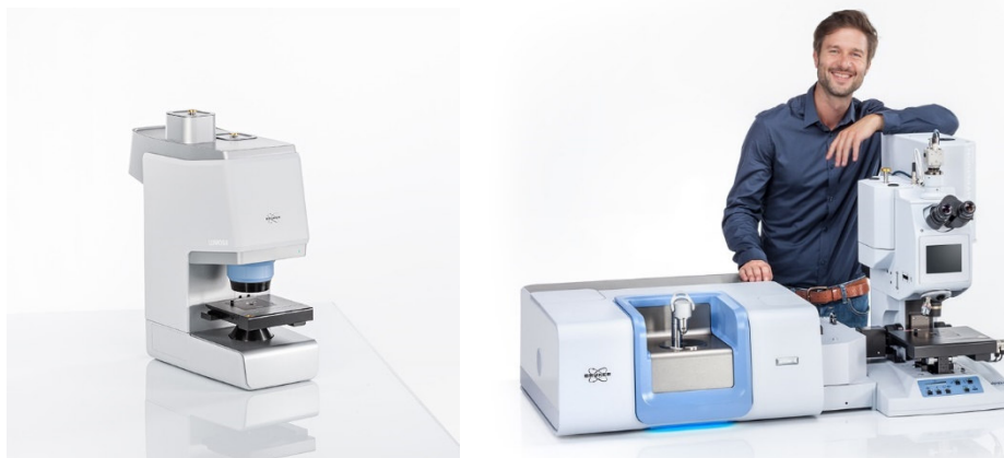
Figure 2: Bruker microscopes, left: Lumos II, right: Hyperion attached to an Invenio spectrometer
