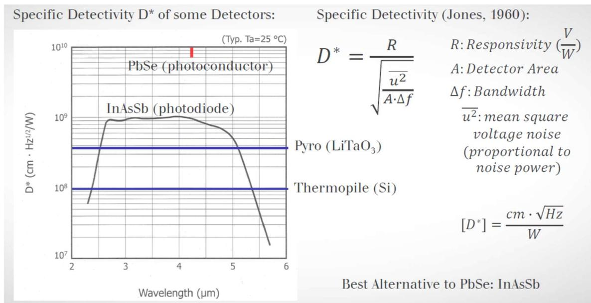
The alternatives to PbSe photoresistive detectors are thermal pyroelectrical detectors, thermal thermopile detectors and InAsSb photodiode detectors. It can clearly be seen that PbSe is technically superior to the known alternative materials (detectivity D\* almost an order of magnitude higher). So a 1:1 substitution of PbSe with another material yielding the same performance is to our present knowledge not possible.
