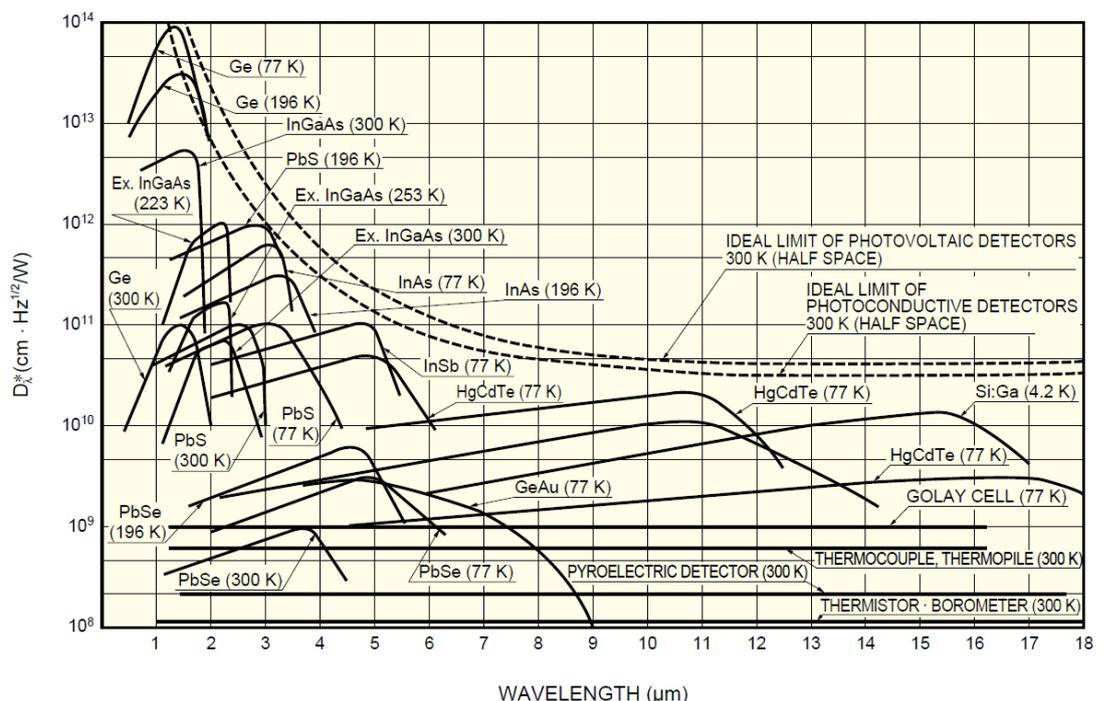
Figure 2. Spectral response characteristics of various infrared detectors
