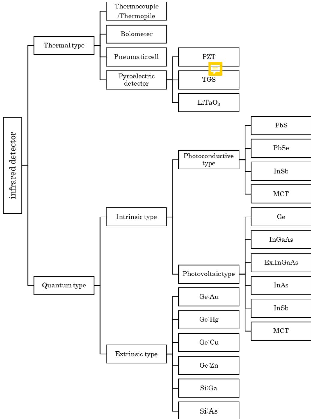
Figure 1. Classification of infrared detectors
