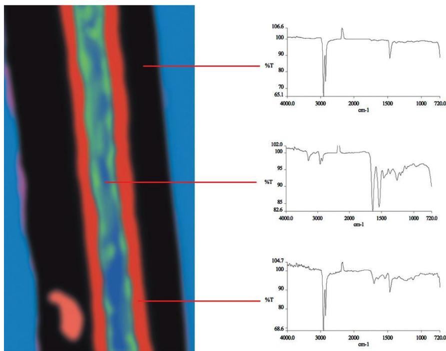
**Figure 4 Polymer laminate showing individual layer of  $<10\mu\text{m}$  thickness**
