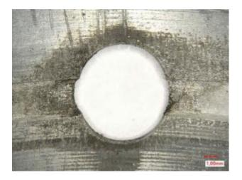
Second test runs with lead free bronze (steel back and CuSn10Bi8Zn3): thermal shock run (no cavitation) however the 1500h release run test is still ongoing.
