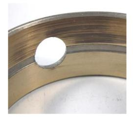
Another EUROMOT member have been completing some testing and evaluations for main bearings for different engine platforms and all future engine programs are striving to be lead free for the powertrain bearings: crank bearings, rod bearings, piston pin bushings (where applicable). There are efforts on some of the current platforms to transition away from the leaded bearings with some platforms being partial lead-free.
