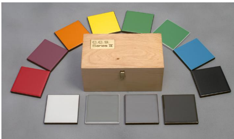
Fig. 1. The set of twelve calibrated reflecting ceramic tiles is produced by CERAM®
