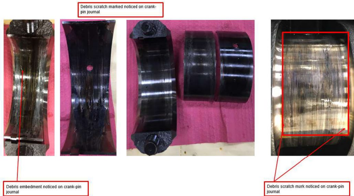
Figure 16 Lead-free test 1, cylinder 4 filled with debris from fracture joint (1.00 mm; qty = 5 chips)
