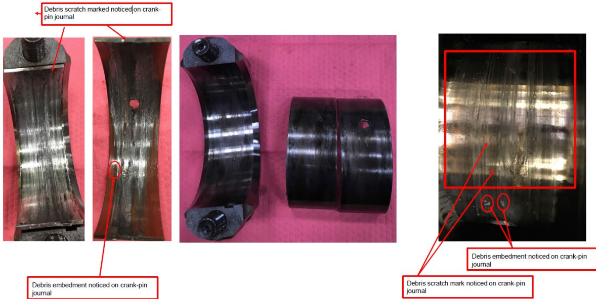
Figure 16 Lead-free test 1, cylinder 4 filled with debris from fracture joint (1.00 mm; qty = 5 chips)
