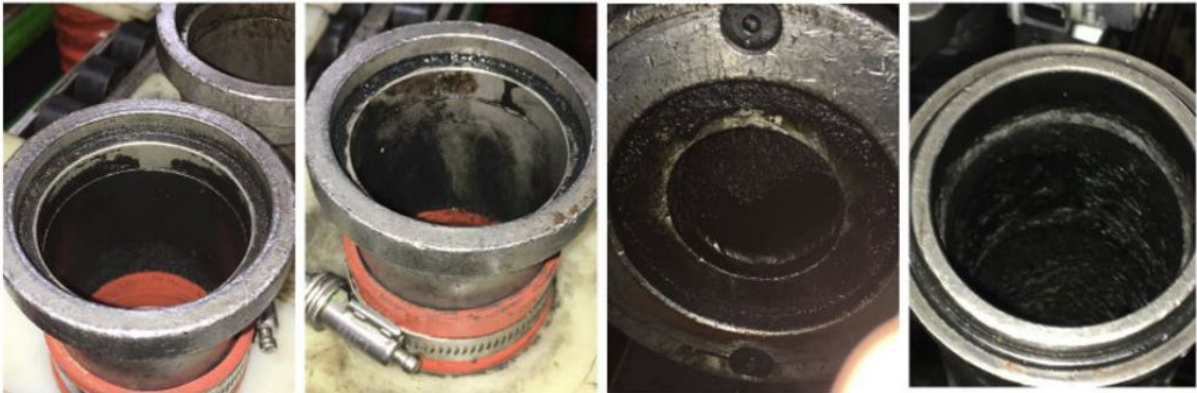
Figure 24 Bearings showing contamination after operation and service in dirty environments
