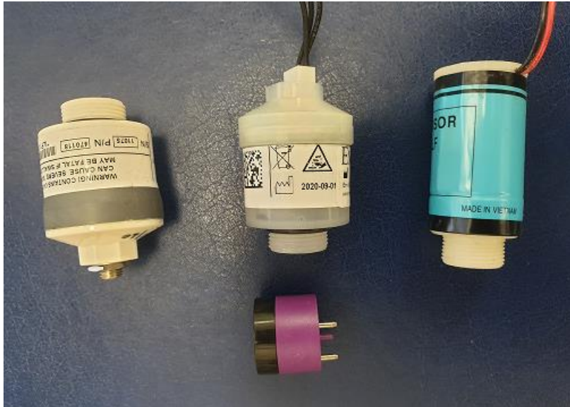
Figure 6 Comparison of an Alphasense O2A2 (which is the same dimensionally as Alphasense A series and elsewhere as 4 series) sensor and the galvanic lead free partial pressure sensors
