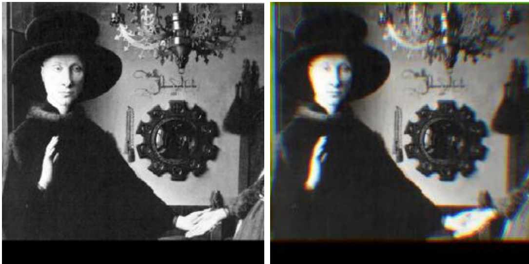
Figure 27. Photographs obtained with lead-based glass lens (left image) and lead-free glass lens (right image). Note colour fringes on right image which is also blurred.
