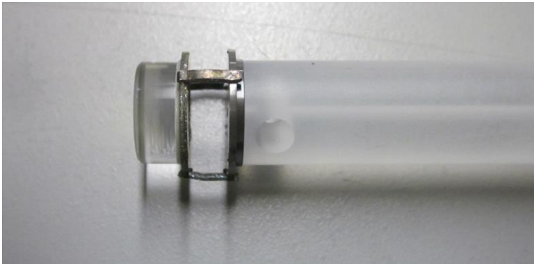
Example of metal attached to laser tube. The glass frit used for this attachment is not visible.
